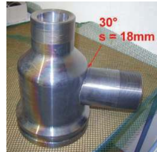
Angle valve body with 3D saddle contour, 30 mm wall thickness
