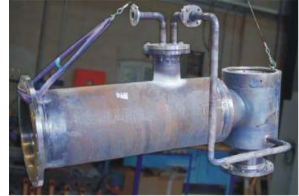
Combined housing with 2D and 3D weld seams
