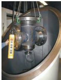
Canister filter DN 200, 3D and circumferential welds
