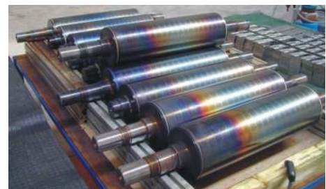
Edge layer hardening and welding of sockets in one clamping position
