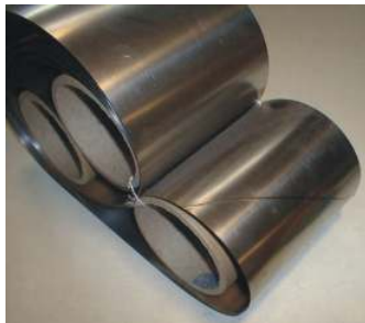
Electron beam welding of conveying belts, 0.2 mm
