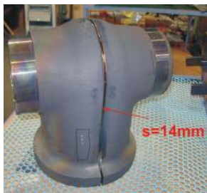
Gate valve bodies made from welded shells DN 150 s = 14\text{mm}
