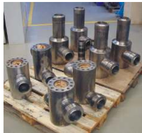
Angle valve body for nuclear valves, 3D socket welding
