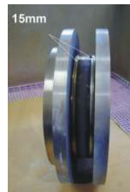
Circumferential weld seam DN 300, 15 mm deep, 15Mo3 15mm
