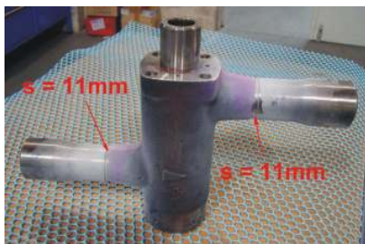
Electron beam welding of sockets from 13CrMo44 s = 11\text{mm}
