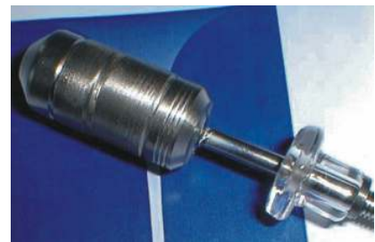
Electron beam welded tungsten anodes
