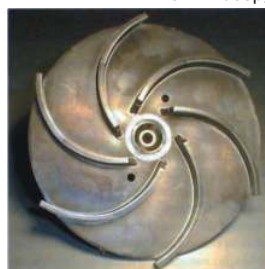
Pump impeller with 3D welds
