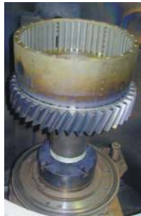
Splined shaft for a pinion carrier, finally welded
