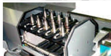
Automatic tool changer with 10-fold plate magazine or 12-fold pick-up-magazine.
