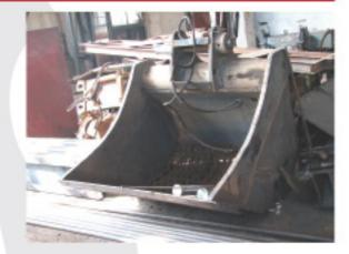
The arrows and buckets for excavators are made of wear-resistant steel, which ensures longer operations.
