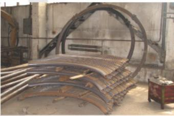
The mine-metal roof support is used to reinforce tunnels for subways, highways and in the mining industry .The Company is doing metal bending with extremely high accuracy in the bending process.
