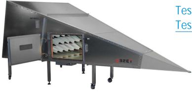
Testing the immunity to radiated electromagnetic disturbances Testing equipment - GTEM Cell (Gigahertz TEM) – 750 (septum height)
