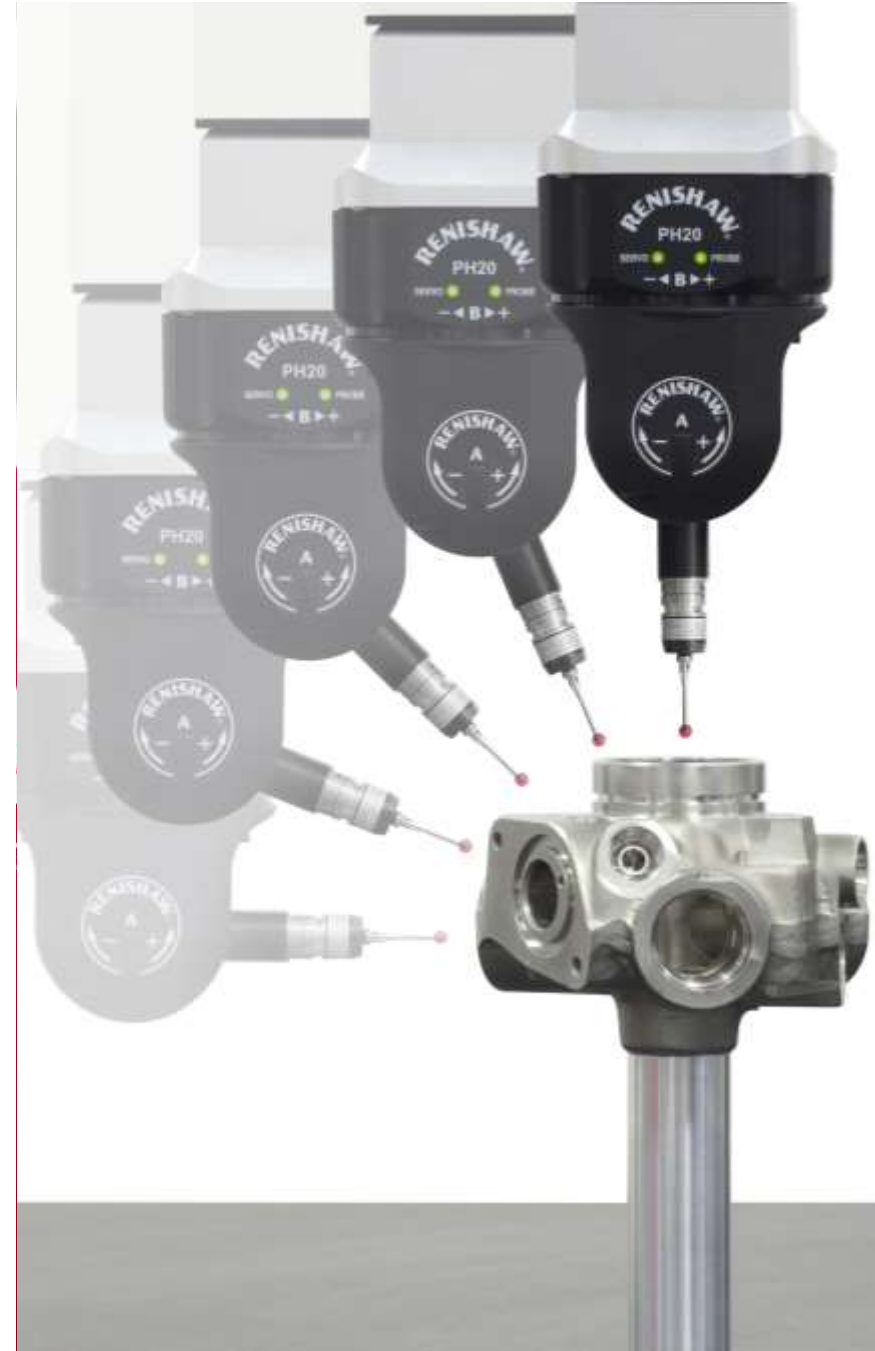
CMM Dimension&Precision X: 700 mm Y: 700 mm Z: 1000 mm 2.3 + L/300 \mu
