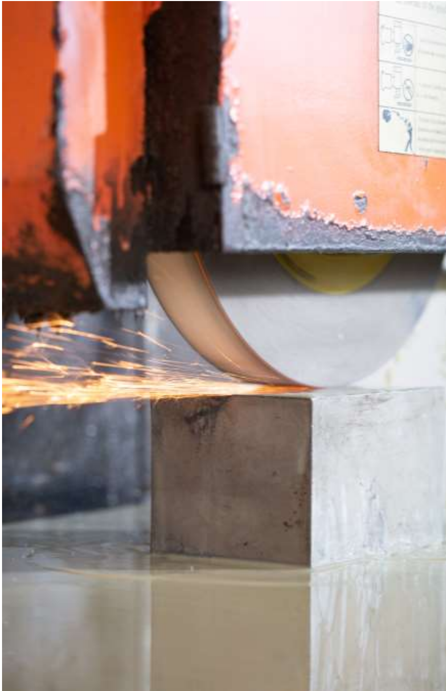
Surface Grinding Dimension X: 1000 mm Y: 500 mm Z: 500 mm
